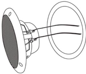
Connect the speaker wires to the speaker
